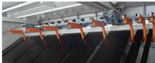
**Lever type pneumatic sheet support system (optional)**
